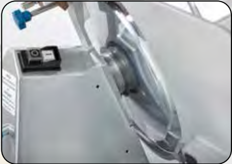
Switches mounted on top to reduce failures
