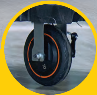
Motorized drive wheels reduce the effort needed to move up to 1,000 lbs.
